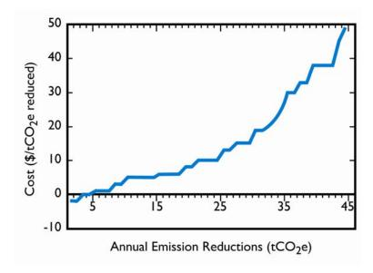
The curve shows the estimated unit cost ( $\frac{1}{CO_2}$  equivalent) and annual emission reduction (t CO<sub>2</sub> equivalent) for emission reduction and sequestration options for a given region and date arranged in order of increasing unit cost.
