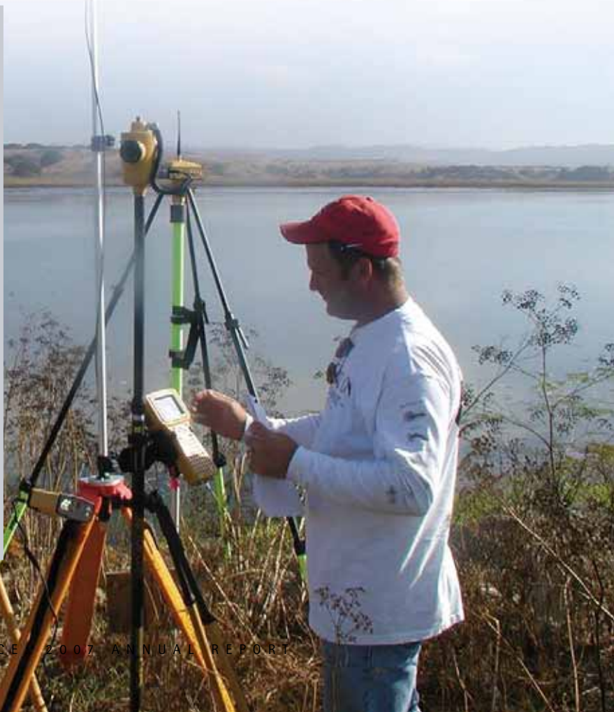
The Global Positioning System revolutionized surveying, providing latitude, longitude, and height information more quickly, inexpensively, and accurately than was possible by traditional surveying methods.
