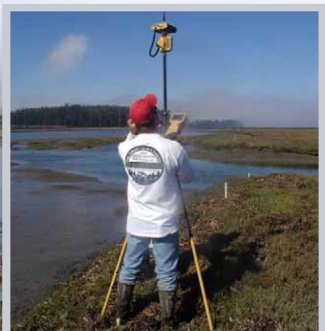
The Global Positioning System revolutionized surveying, providing latitude, longitude, and height information more quickly, inexpensively, and accurately than was possible by traditional surveying methods.
