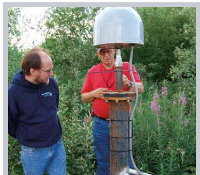
NOS employees inspect a Continuously Operating Reference Station (CORS) in Alaska. CORS sites help NOS provide precise positioning services as well as a number of other scientific and engineering applications.
