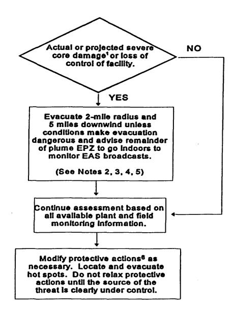
Severe core damage is indicated by (1) loss of critical functions required for core protection (e.g., loss of injection combined with a LOCA); (2) high core temperatures(PWR) or partially covered core (BWR); (3) very high radiation levels in area or process monitors.
