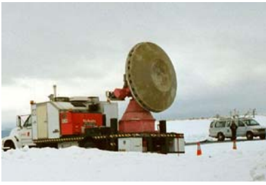
The OU Doppler-on-Wheels and the NSSL mobile laboratory take measurements of a snowstorm in Idaho during IPEX.
