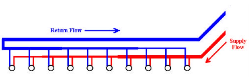
**Fig. 3.7. Design of supply and return lines.**
