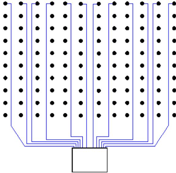
**Fig. 3.5. Ground heat exchanger pattern.**
