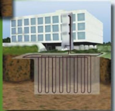
Matrix of ground heat exchangers in vertical bores
