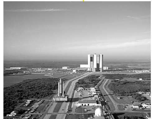
The "crawler" carries a space shuttle to the launch pad.
