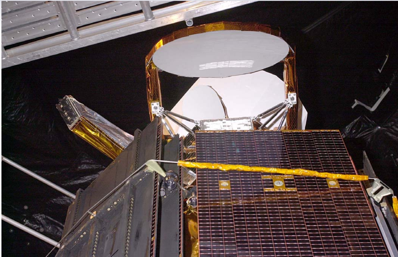
S/N02 SSMIS Sensor on F16 DMSP Spacecraft on Launch Pad at VAFB
