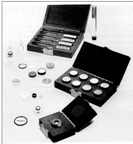
Figure 5.1 Calibration and Reference Sources. Calibration and reference sources may not need evaluation and registration by NRC or Agreement States.
