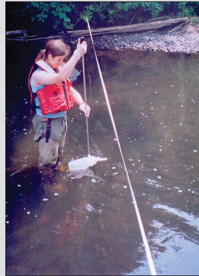
Collecting a depth- and width-integrated water sample in a river in Massachusetts. (Photograph by J.R. Deacon, U.S. Geological Survey.)
