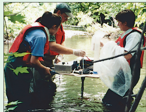
Collecting a ground-water sample beneath the streambed of the Aberjona River. (Photograph by K.W. Robinson, U.S. Geological Survey.)
