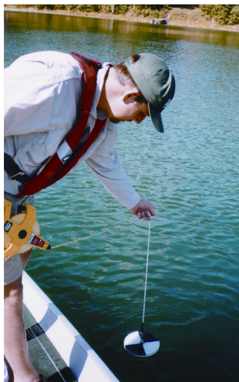
Figure 8. USGS scientist measuring the transparency of lake water using a Secchi disk. (Photograph by Rick Hubbell; U.S. Geological Survey.)
