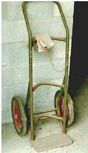
Figure K-4 - Cylinder Cart, Not Allowed
