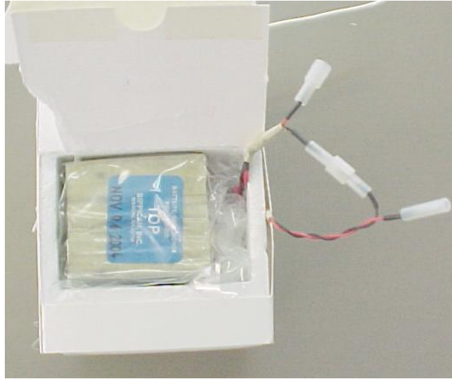
Figure N-14-Connect the Wires First (Inside the Radiosonde).
