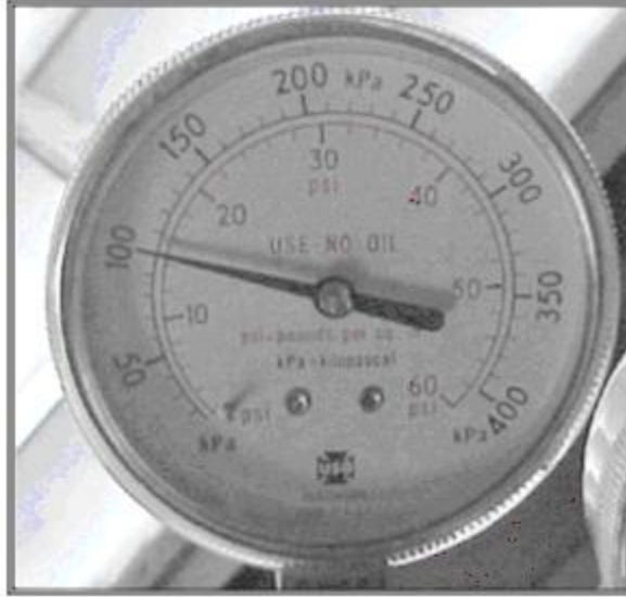
Figure D-5 - Gauge Measuring Hydrogen Line Pressure
