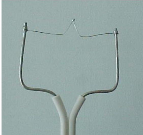
Figure N-4 – Temperature Sensor
