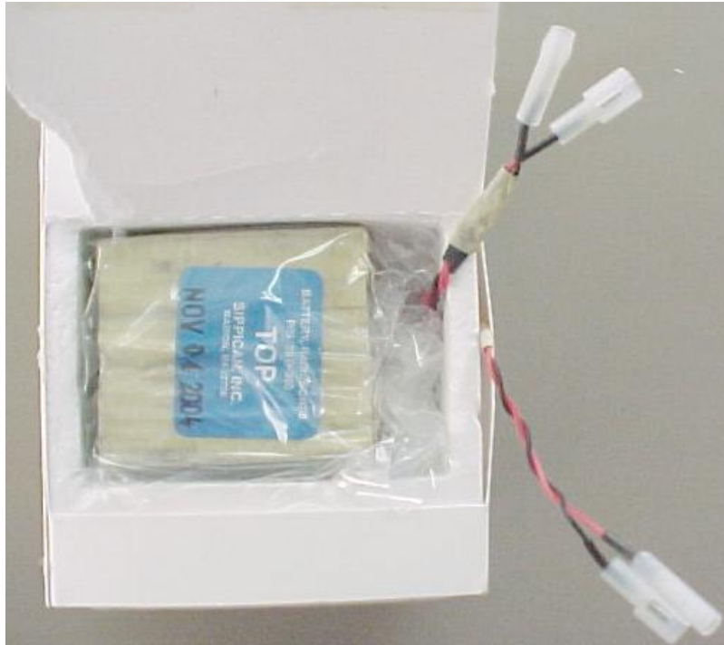
Figure N-12 – Twist Battery Wires
