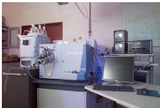
High-resolution hybrid Linear Trap Quadrupole/Orbitrap™ Mass Spectrometer located in EMSL's Aerosol Chemistry Laboratory.
