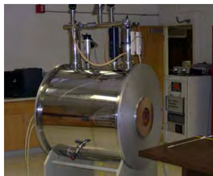
Figure 10. Horizontal-bore 2-T magnet.
