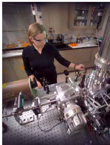
Figure 7. The second-generation single particle laser ablation time-of-flight mass spectrometer offers users the versatility of laboratory studies and field campaigns.
