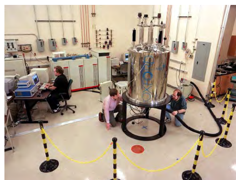
Figure 6. Varian NMR System 500-MHz wide-bore NMR spectrometer.
