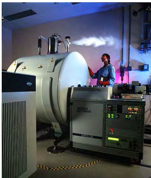
Figure 3. 150-mm-bore, actively shielded 9.4-T FTICR instrument.
