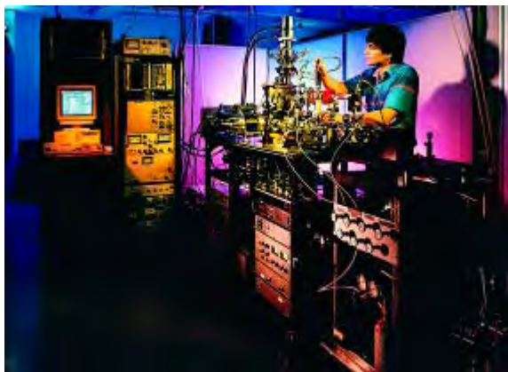
Figure 4. Electron-stimulated surface reaction apparatus is used to study non-thermal reactions that occur on surfaces or at interfaces.
