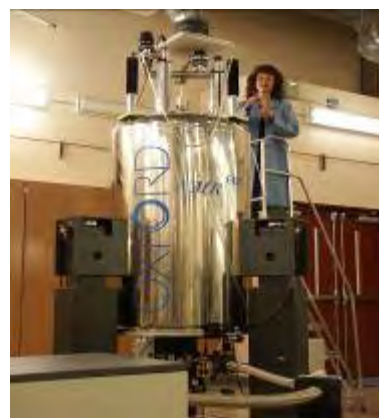
Figure 4. Varian INOVA 600- MHz NMR spectrometer with Cryoprobe.
