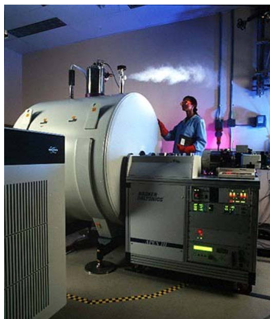
Figure 3. 150-mm-bore, actively shielded 9.4-T FTICR instrument.
