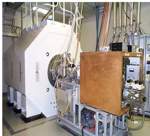
Figure 2. Wide-bore, passively shielded 11.5-T FTICR MS.
