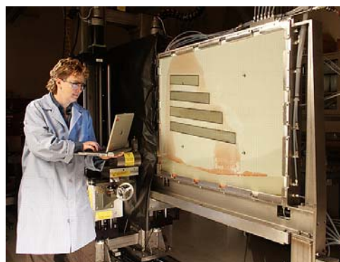
Figure 1. EMSL researchers test theories of flow and transport. The study coupled processes involved with microbial, reactive chemical, NAPLs, colloid transport, or test subsurface remediation scenarios using the Subsurface Flow and Transport Laboratory.
