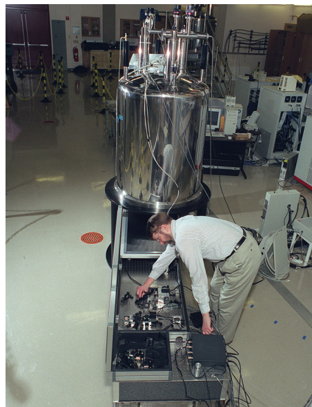
Figure 2. Combined instrument that allows fluorescent optical microscopes and magnetic resonance microscopes to focus on the same samples at the same time.
