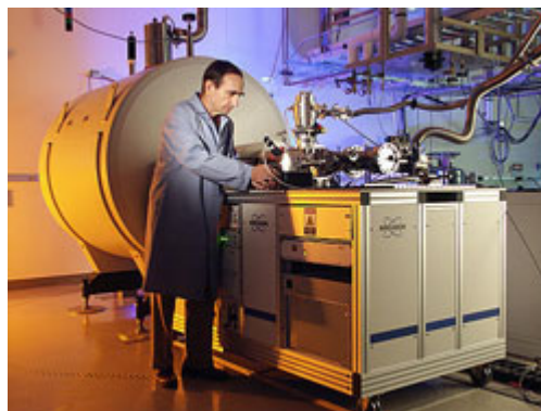
Figure 7. Harold Udseth and the new 12-tesla magnet equipped on a Fourier-transform ion cyclotron resonance mass spectrometer.
