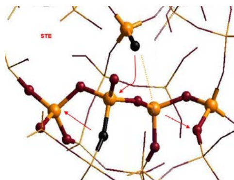
Figure 1b. Exciton-induced damage process in amorphous silica. Self-trapped triplet state exciton configuration. A Si-O bond has been broken.
