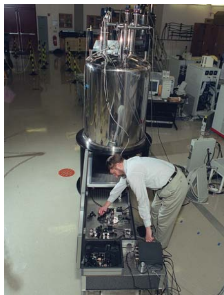
Figure 2. This combined instrument allows fluorescent optical microscopes and magnetic resonance microscopes to focus on the same samples at the same time.
