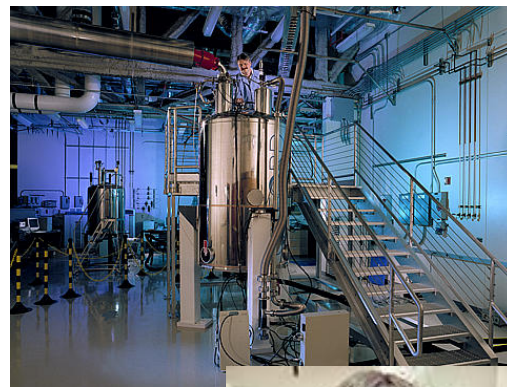
Above: EMSL's 800-MHz NMR system used in the research. Right: Valérie Copié.
