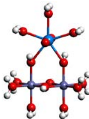
Atomic cluster used to calculate the stability of uranium as a function of its oxidation state. Fe atoms (purple) are in the geometry of Fe in magnetite. The U atom is blue, O atoms are red, and H atoms are white.
