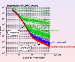
Emergence of the Error-Floor is a caveat of BP Instanton (optimal fluctuation) method Tanner code. Gaussian channel. Tanner code. Laplacian channel. Linear Programming Decoding
