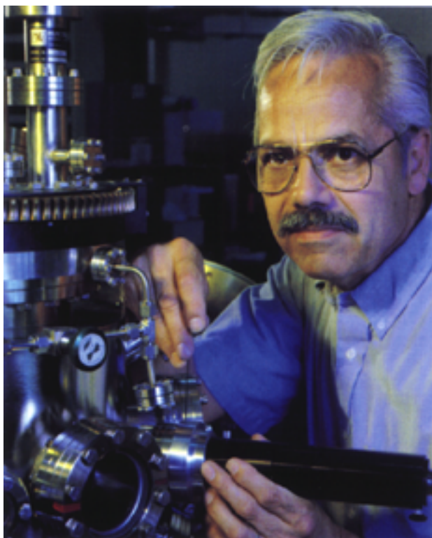
George Castro of IBM's Almaden Research Center led the commissioning of a photo-electron microscope at the Advanced Light Source that produces images of solids and their surfaces by means of the electrons emitted when a sample absorbs X-rays.
