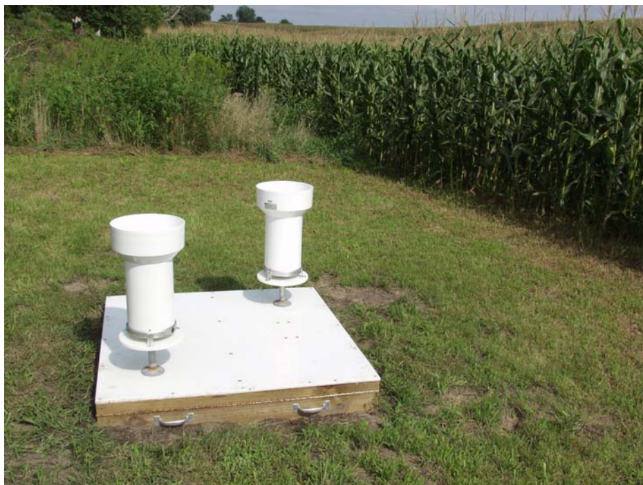
Figure E.5. Double rain gauge platforms installed at the Iowa City, Iowa, network.
