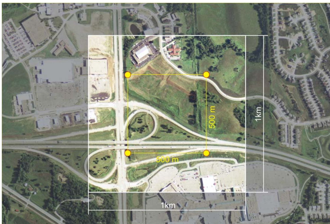
Figure E.7. Ground reference rain gauge cluster configuration that results in point-to-area variance reduction of over 90% assuming exponential correlation function with the correlation distance of 5 km or more.
