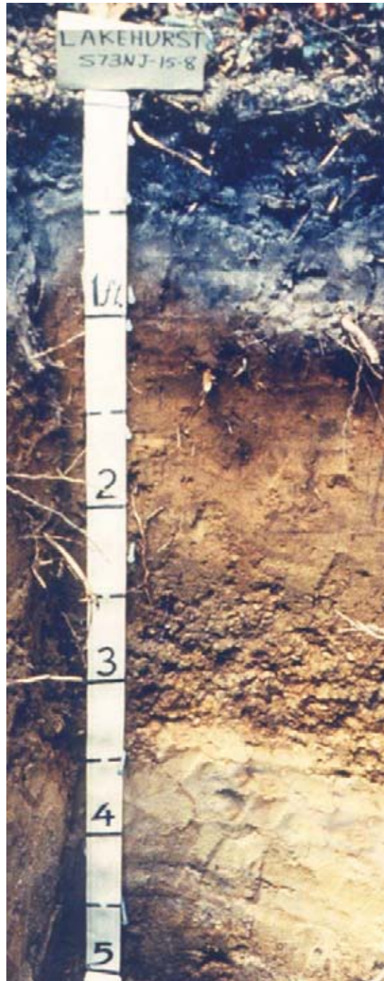
Figure 14.—A profile of a Lakehurst soil. Lakehurst soils formed in sandy fluviomarine sediments deposited over marine sediments.
