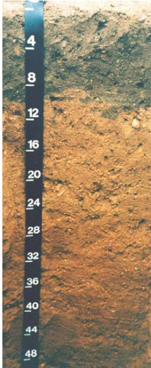
Figure 12.—A profile of a Downer soil. Downer soils formed in loamy or gravelly fluviomarine sediments.
