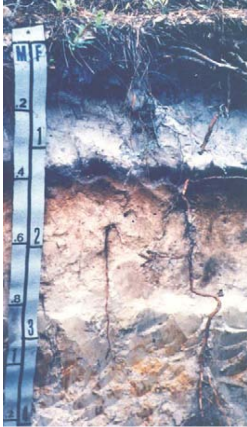
Figure 10.—A profile of an Atsion soil. A thin, dark Bh horizon is below a depth of about 1.2 feet. Atsion soils formed in sandy fluviomarine sediments. They have a seasonal high water table at or near the surface for long periods.
