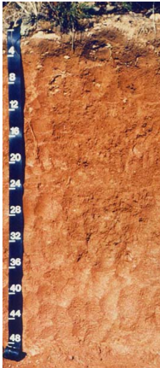
Figure 16.—A profile of a Sassafras soil. Sassafras soils formed in loamy or gravelly fluviomarine sediments, or both.
