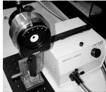
Figure 9. Broad band device for Size-of-Source Effect measurements by the central obscuration method
