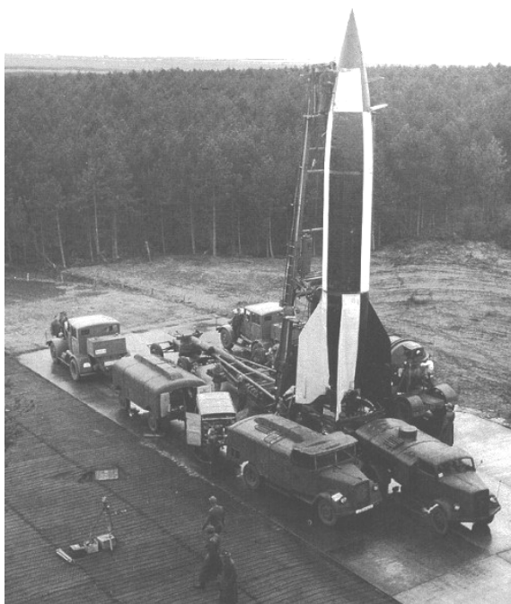
FIGURE 6 —Photo from Operation Backfire showing some of the equipment required to operate the V-2.
