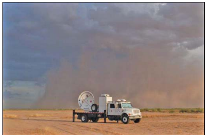
Figure 8: Photograph of one of the two SMART radars during a downdraft haboob event in Arizona. One of the SMART radars will soon be upgraded with dual-polarization capability allowing many new research areas.
