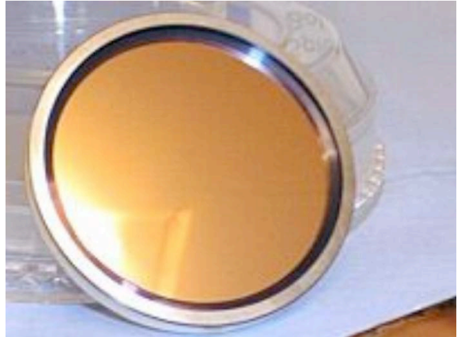
Figure 8.4: Photograph of a quasi-optical metal-mesh low-pass filter (courtesy of Peter Ade).
