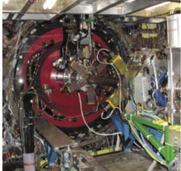
CLEO DETECTOR CLEO detects, measures and analyzes electron-positron collision events generated by CESR.
