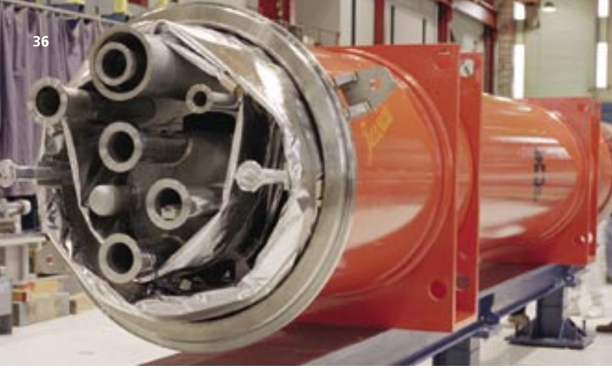
Above (L-R): 1) Superconducting quadrupole magnet, built at Fermilab for the Large Hadron Collider at CERN. Credit: Fermilab 2) Laser source producing polarized electrons for the SLAC accelerator. Credit: SLAC
