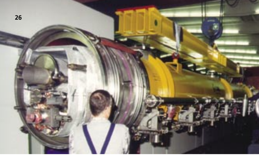
Above (L-R): 1) Superconducting accelerator structures at the TESLA test facility at DESY in Hamburg, Germany. Credit: DESY 2) Waveguides for linear collider under development at the Accelerator Test Facility at KEK in Japan. Credit: KEK
