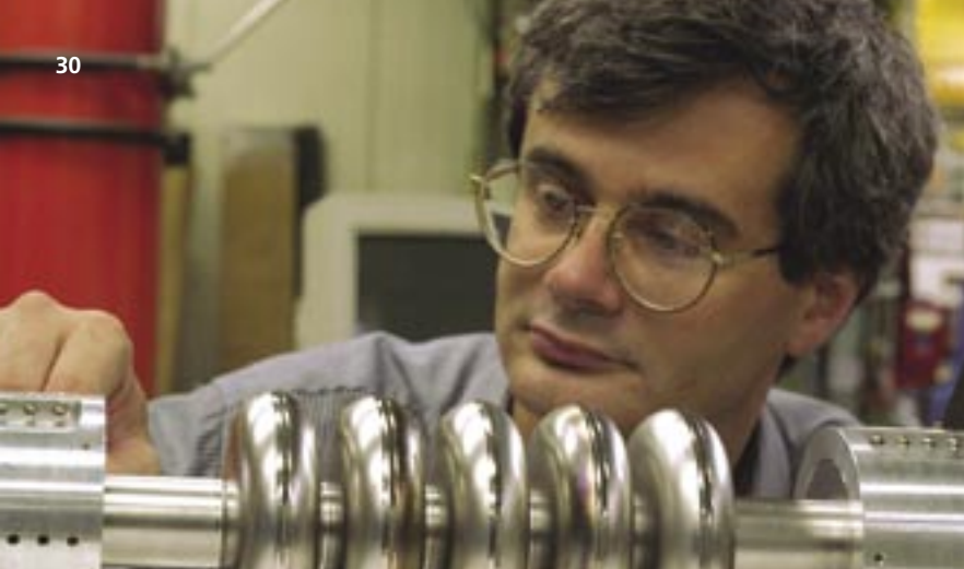
Above (L-R): 1) Fermilab physicist Leo Bellantoni with superconducting radio frequency cavity. Credit: Fermilab 2) Machined copper disks prepared for X-band radio frequency cavity. Credit: KEK
