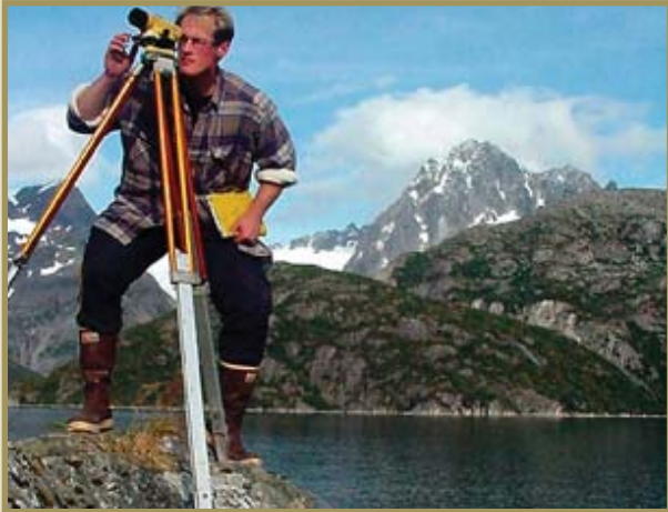
Erik Oppegard performing leveling to tidal bench marks, Striation Island, Kenai Fjords National Park, Alaska, in 2000. Note: In 1950, this area was under about 1,000 feet of glacial ice. Credit: LCMF, Inc.
