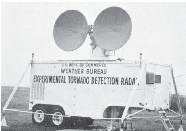
FIG. 2. USWB's continuous-wave 3-cm Doppler radar with its side-by-side transmitting and receiving antennas used for tornado studies in the southern plains during the late 1950s. The unit was converted by NSSL into a pulsed Doppler radar in 1964. [USWB photo.]
