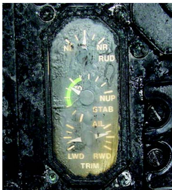
Figure 4. The accident airplane's pitch trim position indicator display, as documented postaccident.
