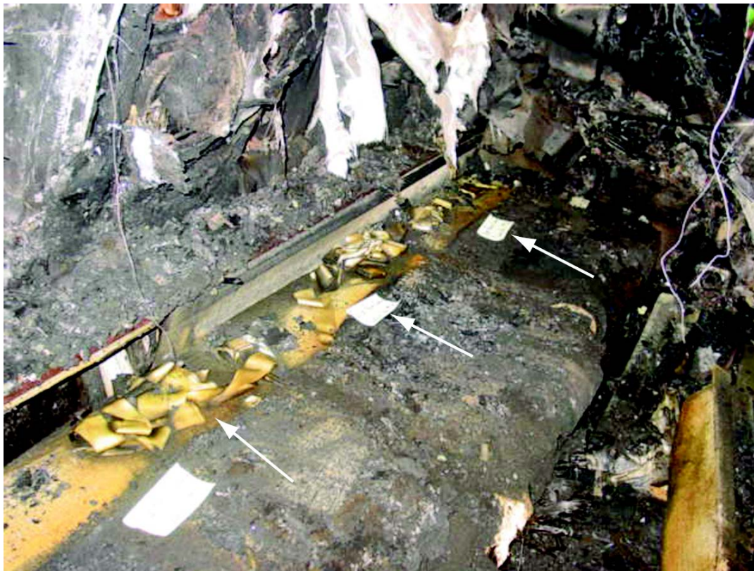
Figure 5. The side-facing, three-passenger divan from the accident airplane with the burned seat cushions removed. Note: the arrows indicate the row of folded seatbelts that were found beneath the seatback cushions.
