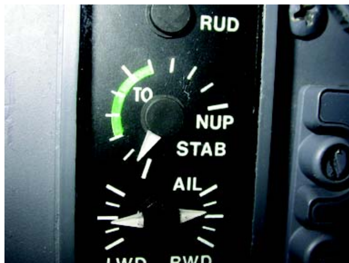
Figure 3. Photograph of a CL-600 pitch trim position indicator similar to that in the accident airplane.
