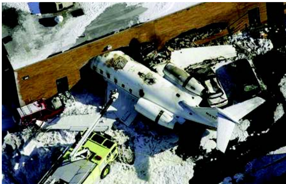
Figure 6. The accident airplane, the impacted building and several impacted vehicles, and the HRET/skin-penetrating nozzle-equipped firefighting vehicle.
