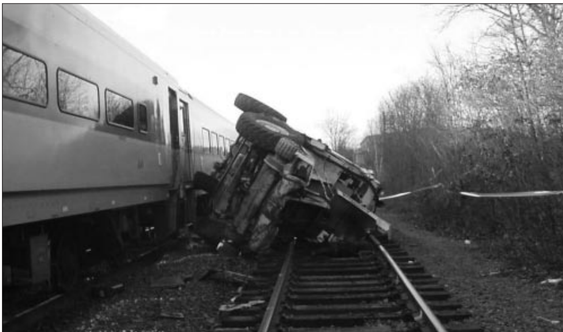
Figure 3. Damaged track maintenance vehicle.
