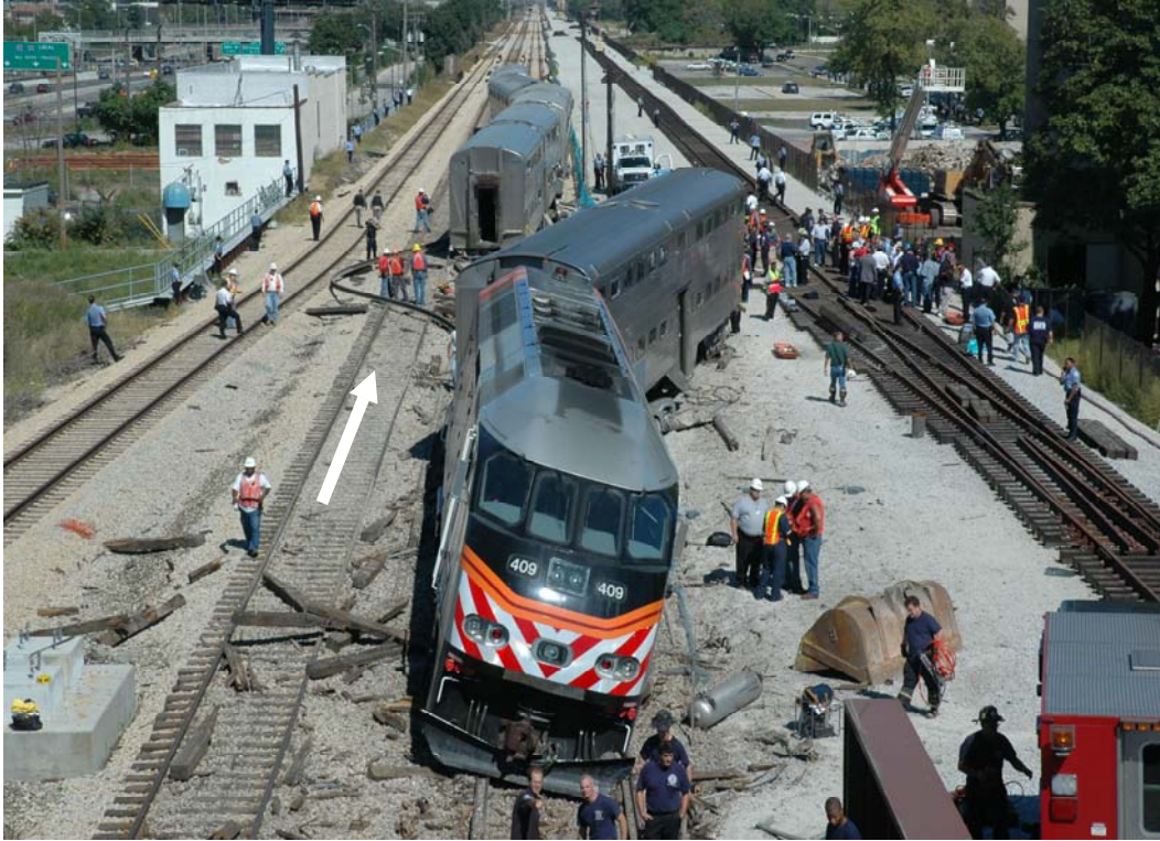
Figure 1. Train after derailment. (It was operating in push mode and traveling in the direction of the arrow.)
