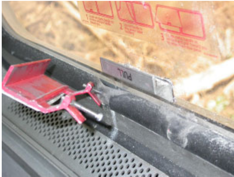
Figure 11. Emergency window handle that partially pulled free from rubber grommet.
