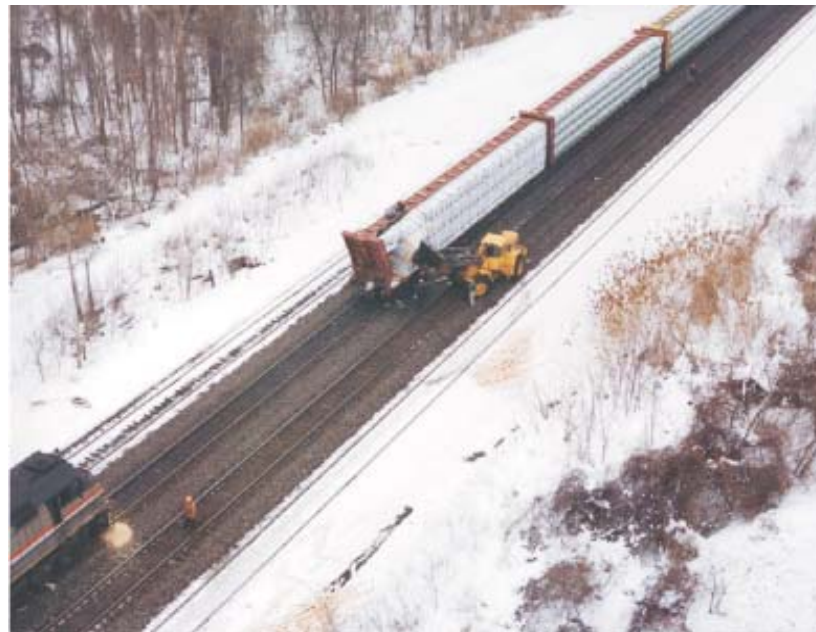
Figure 4. Postaccident positions of the end of the CSXT freight train and the lead Amtrak locomotive unit.
