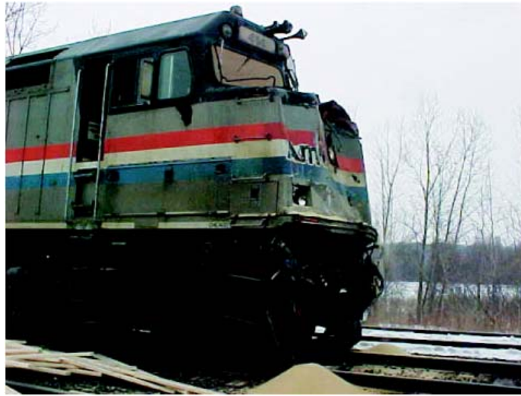
Figure 6. Damaged lead locomotive of Amtrak train 286.
