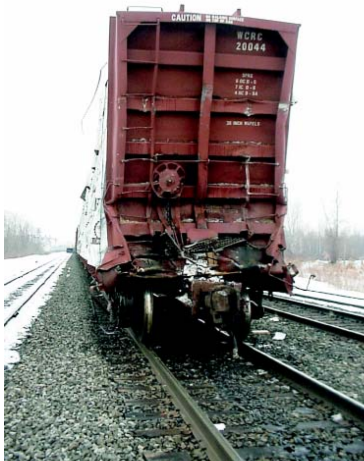
Figure 5. Damaged rear freight car of CSXT freight train Q620.
