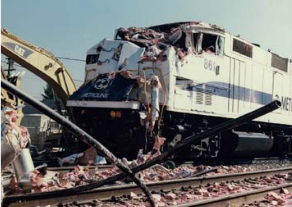
Figure 12. Postcollision view of locomotive. (Photograph source: Glendale, California, Police Department.)
