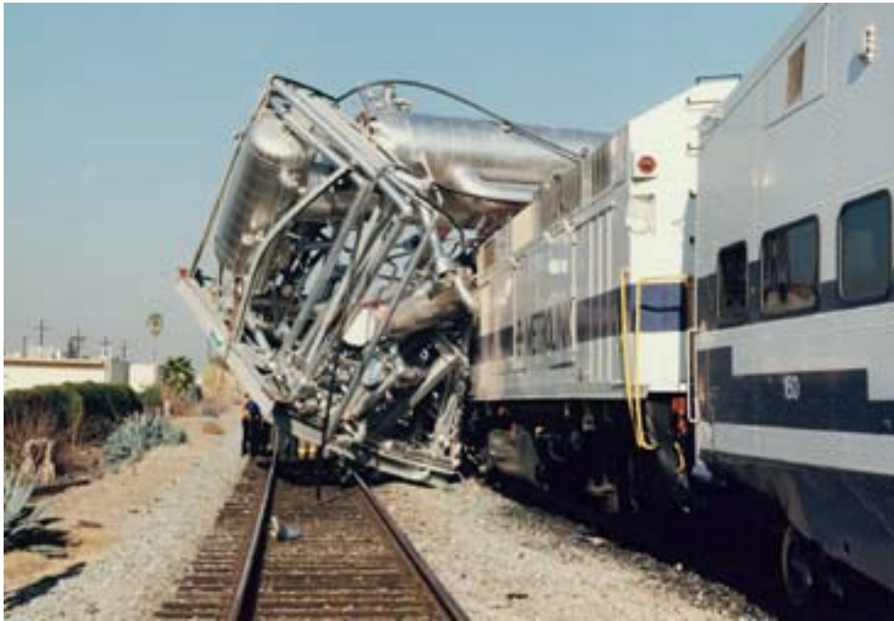
Figure 11. Postcollision view of condenser and train. (Photograph source: Glendale, California, Police Department.)
