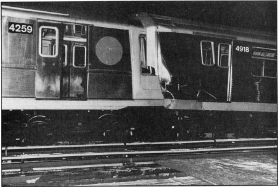
Figure 3--Rear car 4259 of B train penetrating lead car 4918 of M train.
