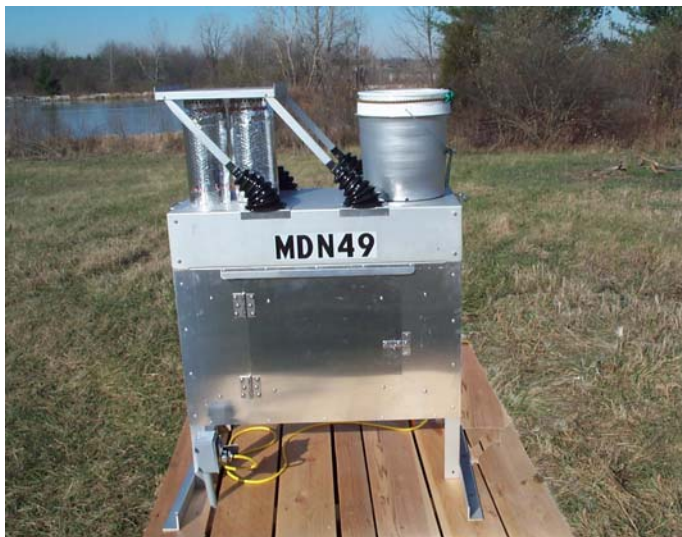
Figure 5. Automated precipitation collector and rain gage for monitoring station.
