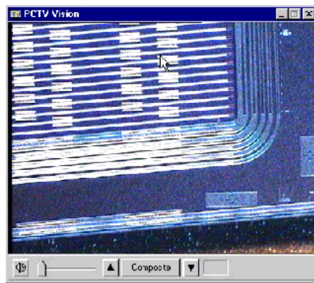
Figure 2.7: The corner of a silicon microstrip detector . The guard rings structure surrounds the strips region.
