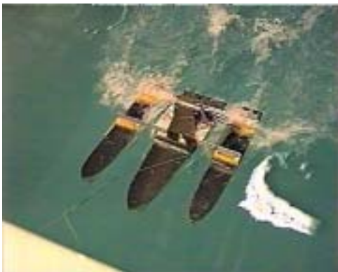
Figure 9. Trimaran #2 in the tow tank.
