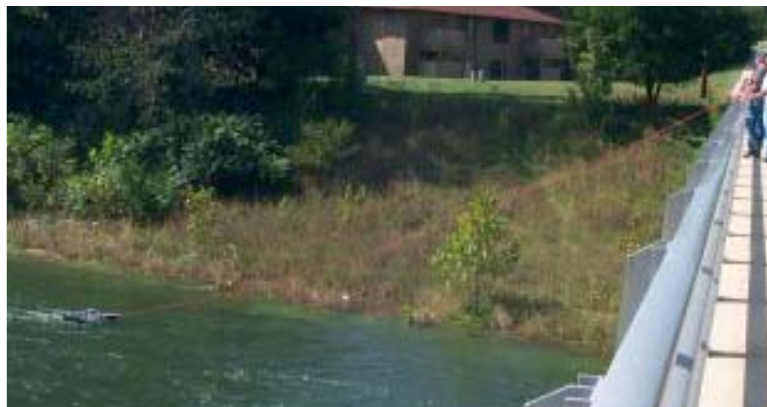
Figure 13. Monohull tethered platform being field tested by the U.S. Geological Survey.
