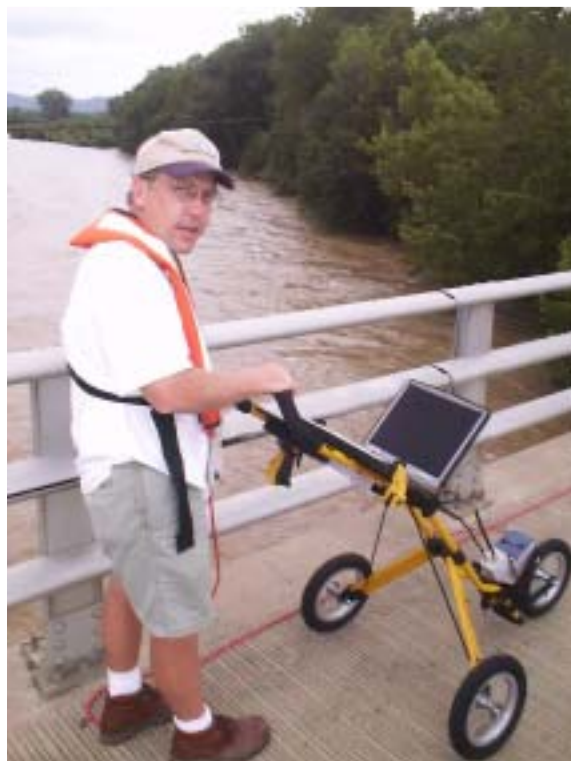
Figure 14. U.S. Geological Survey personnel and the personal computers used to collect data during an unmanned tethered-platform acoustic Doppler current profiler discharge measurement.
