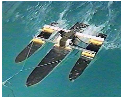
Figure 10. Trimaran #3 in the tow tank.
