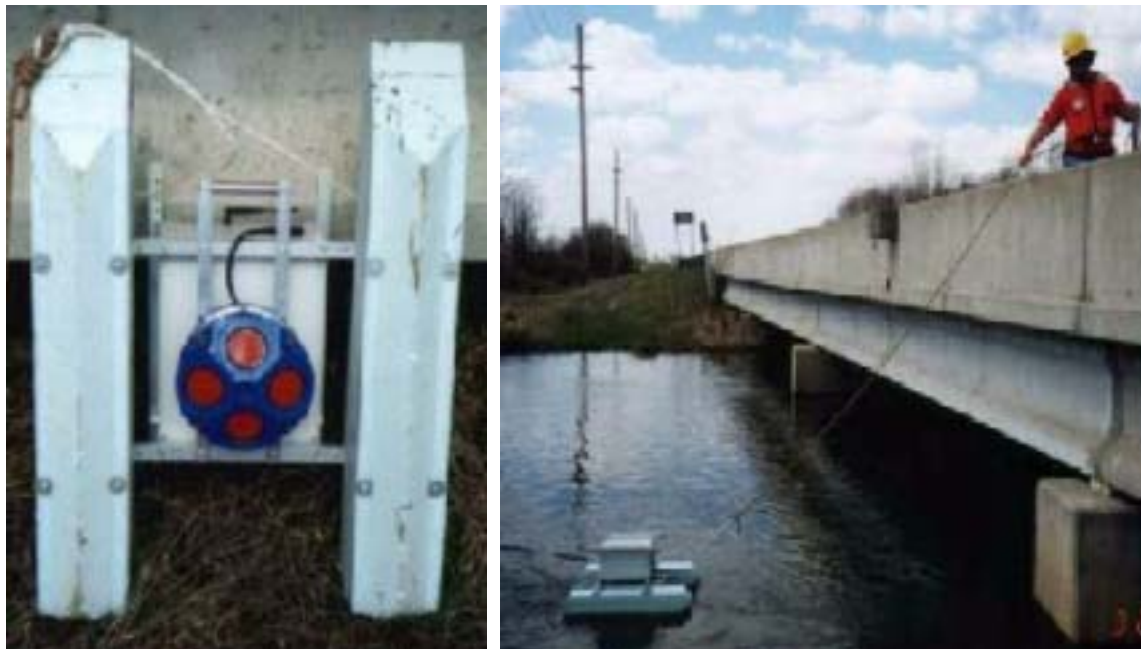
Figure 2. Original U.S. Geological Survey Indiana District prototype acoustic Doppler current profiler (ADCP) tethered platform.
