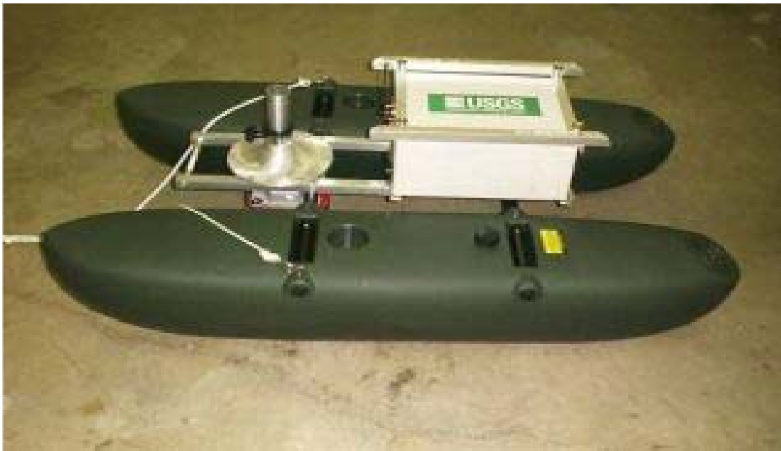
Figure 3. Hobie Floatcat modified for use with an acoustic Doppler current profiler.
