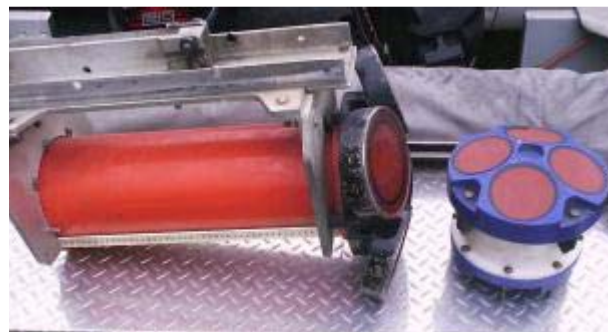
Figure 1. Comparison of first (left) acoustic Doppler current profiler (ADCP) used by the U.S. Geological Survey Indiana District and a newer model (right) ADCP purchased in 1997.
