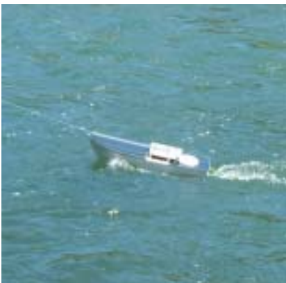
Figure 13. Monohull tethered platform being field tested by the U.S. Geological Survey.
