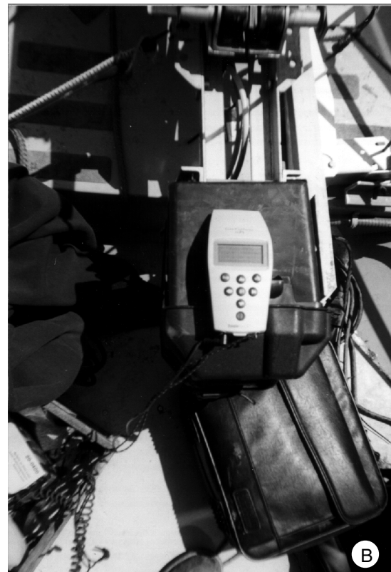
Figure 3. Boat-mounted acoustic Doppler current profiler (A) and global positioning system mobile receiver (B).
