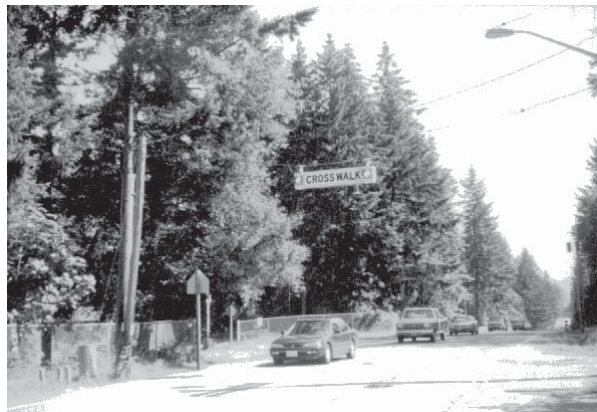
Overhead flashing beacon
