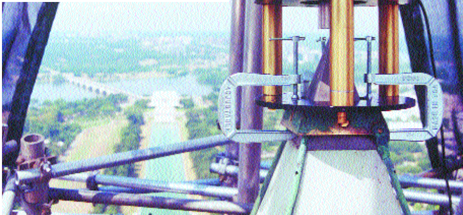
Javad Positioning Systems RegAnt choke ring antenna with Lincoln Memorial in the background.
