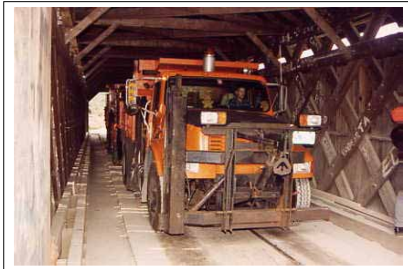
Figure 144. Field tests for deflection measurement comparison against computer prediction—Brown Bridge, Shrewsbury, VT.
