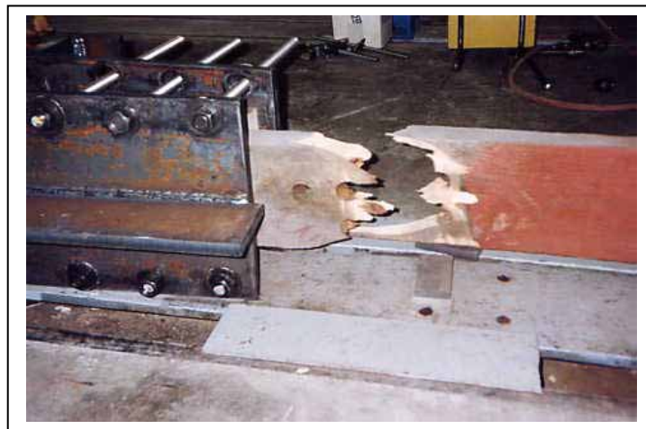
Figure 147. Tensile tests on lattice elements.
