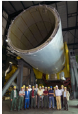
Rotation of the solenoid magnet of the CMS experiment before the insertion into its cryostat. Image courtesy of CERN.
