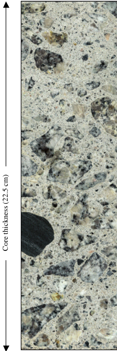
Figure 3.2.15 Polished cross-section of pavement section 13-GA1-5.
